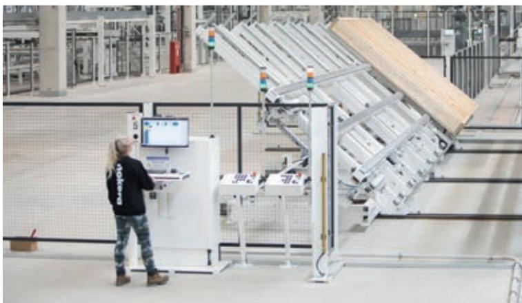
Serial production of a timber module in a NOKERA factory.
