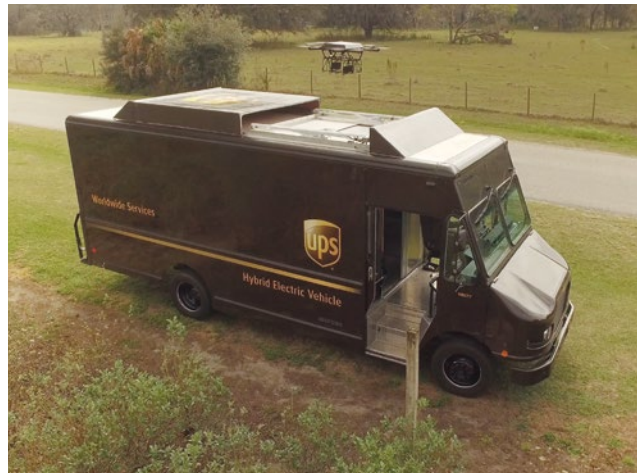
UPS COMBINATION DELIVERY USING VAN AND DRONE (Source: UPS)
